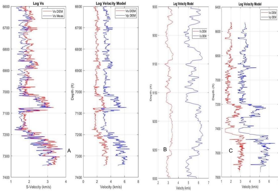
Figure 13. Optimized  $V_p$  and  $V_s$  log results in each well: (A) RZ-14, (B) RZ-09 and (C) RZ-35.
