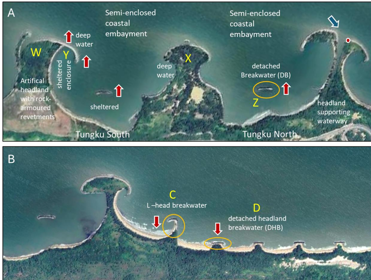
Figure 2. (A) Satellite image of the Tungku coastline (South China Sea) showing artificial rocky structures in two semi-enclosed embayments. W, X, artificial headlands with rock armoured revetments; Y, sheltered part behind curved breakwater; Z, detached breakwater (DB). (B) An adjoining coastline to that above. (C) L-head breakwater and (D) detached headland breakwater (DHB). The names Tungku North and Tungku South are not official. Blue arrow indicates ‘outfall’. Upward arrows indicate high sublittoral species diversity in deeper-water. Sheltered areas subject to sand deposition are indicated. Downward arrows indicate low species diversity, due to shallow water and sand influence on rocky structure. Red circle indicates reference point 4°54’46.7”N, 114°52’46.7”E.
