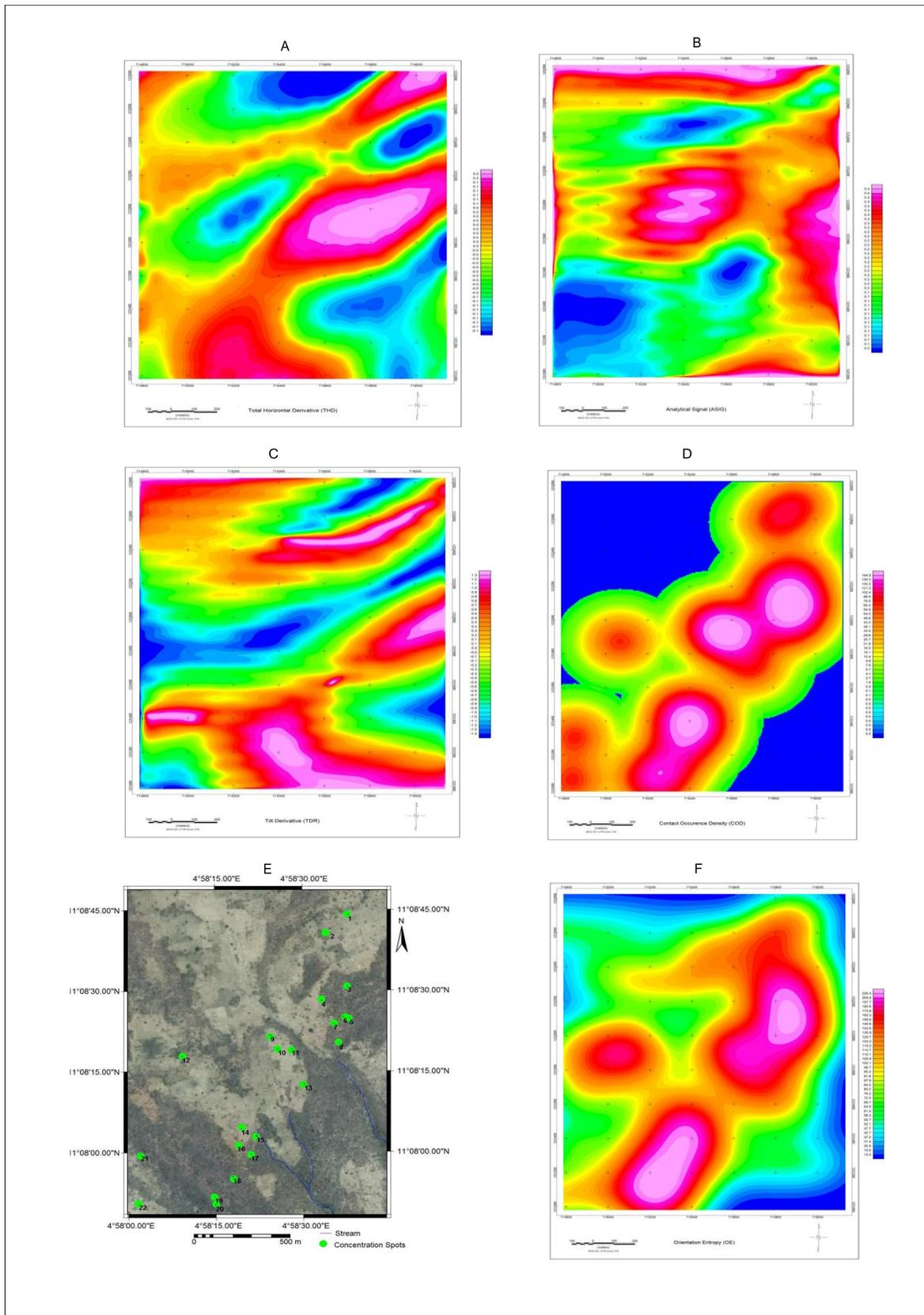
**Figure 9.** Interpreted aeromagnetic data. (A) First vertical derivative, (B) Analytical signal derivative, (C) Tilt derivative grid, (D) Contact occurrence density, (E) Mineral potential map, (F) Entropy map with line of potential mineralization.
