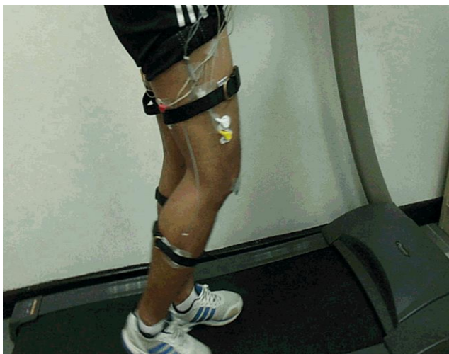
Figure 2. A test subject walking on a treadmill wearing wireless motion and EMG sensors
