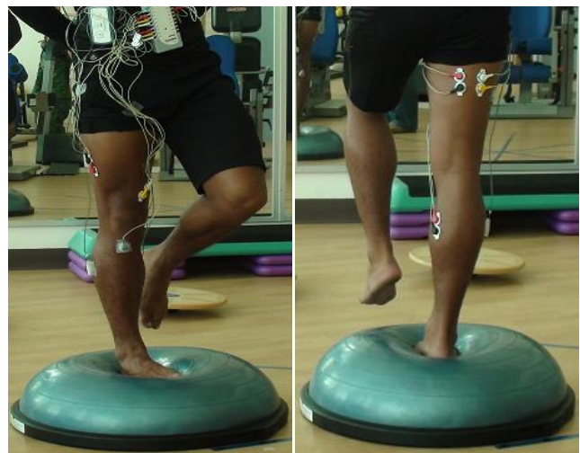
Figure 3. A test subject standing on single leg on a balance trainer wearing wireless motion and EMG sensors - front and back view
